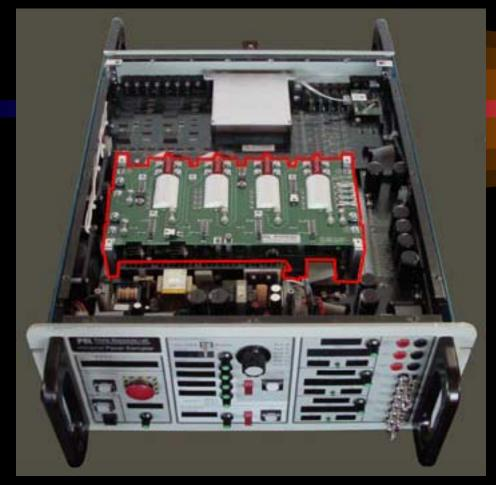
The IGBT Module (insulated gate bipolar transistor)
