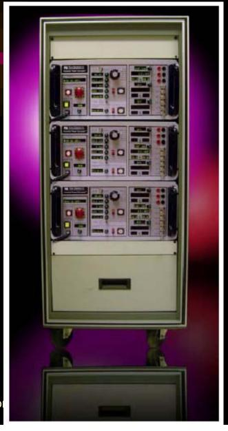
Semiconductor tool manufacturers, and their component suppliers, use the Industrial Power Corruptor to test and design for SEMI F47 compliance and completing data sheet 400 of the SEMI E6 standard.
