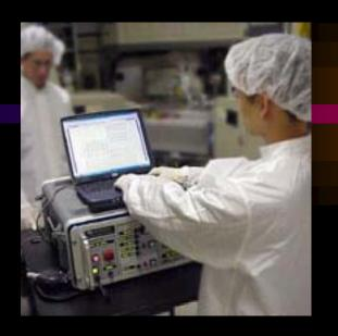
PSL's TestingPartner program is a simple, low-cost way to certify compliance with several standards, including SEMI F47 SEMI E6, and IEC 61000, IEEE 1100. It is based on PSL's latest generation of test equipment, which -- if you allow it to -- lets us look over your shoulder electronically while you perform the tests.
